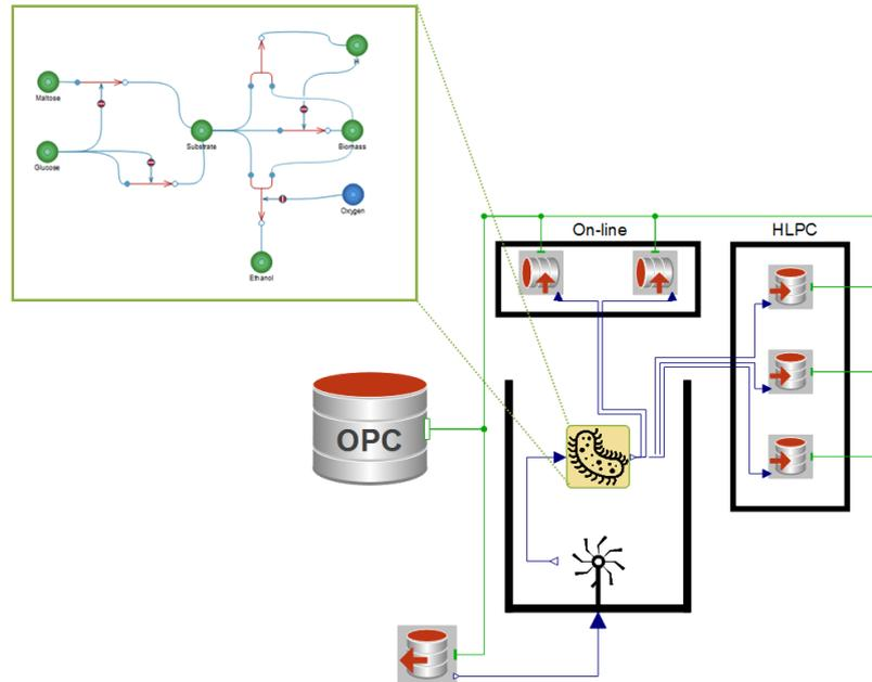
The MPC controller (bottom left) is implemented in the Wolfram Language[3] and controls the amount of oxygen in the batch by adjusting the stirrer speed, while the on-line and HPLC parts communicates with measurement equipment (in this case measurements made in the model). The biochemical model is finally replaced with the real world system.
