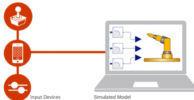
The ModelPlug library allows rapid prototyping of controllers without the need of writing a single line of code, thereby enabling interaction with complex simulation models and easy creation of realistic test scenarios.
